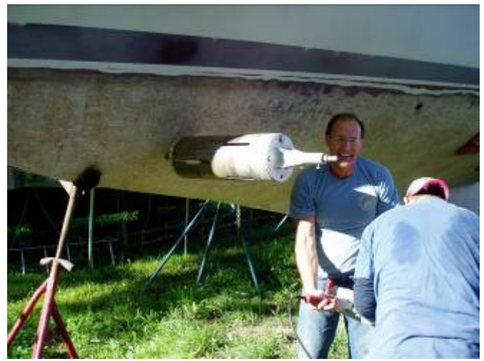
My CSY WO 44 "Dutchess" getting a BOWTHRUSTER details in future editions. That is Joe Molinaro doing the install. Editor
